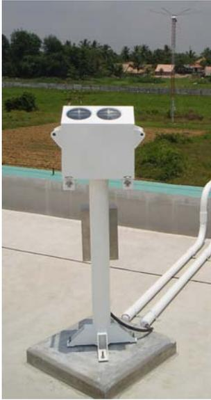
8000-CHS Ceilometer measuring cloud whilst mounted on roof of the equipment room.
